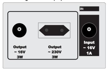
Connect the power cable supplied (polarity --•-+) to the **Output** ~16V 3W socket on the Speed Box SE II and to the power socket on your turntable. The original power supply is then no longer required.
